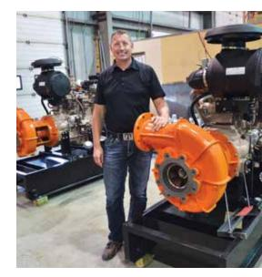
RapidFire & Rescue sources the engines from Frontier Power Products in Calgary, Alberta. Branch manager Joe Leskovjan says the distributorship custom builds the skid-mounted pumping unit with a PowerTech E 4.5L engine and Berkeley pump.
