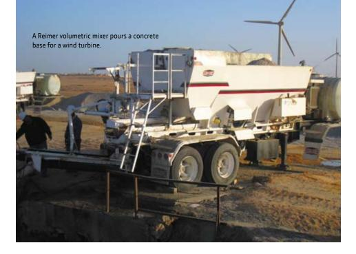
Reimer Mobile Mixers produce up to 57 cubic meters (75 cu. yds.) of concrete per hour and are designed and built to run continuously. "When you're mixing concrete at higher volumes at lower slump, at high production rates, you need an engine that can hold up to that kind of load and pressure," explains Steven. "We are happy with the torque curve of the John Deere engines, because they hold the load right where you need it.
