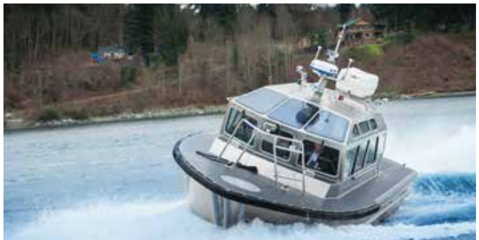
Tymac’s new water taxi, Tymac Wave, demonstrates agility with twin PowerTech 6090SFM85 marine engines. Photo credit: Tremain Media Inc.
