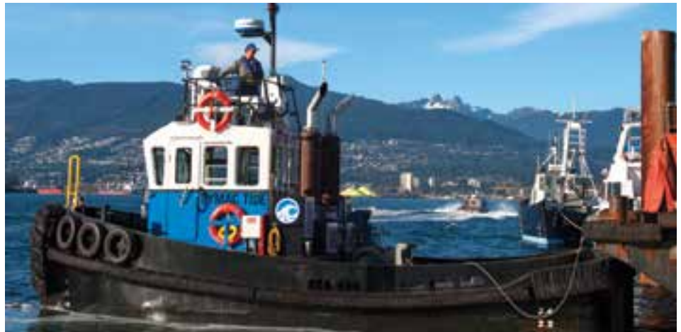
Tymac Tide pushes barges with twin 272-kW (365-hp) PowerTech 6135AFM75 marine engines.
