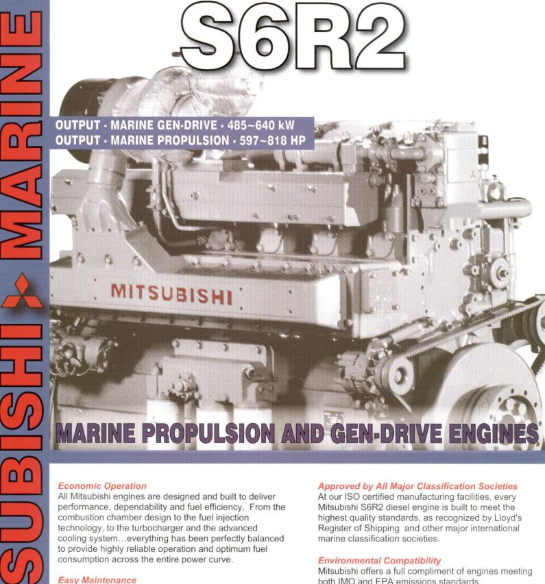
With Mitsubishi's S6R2 marine engine, maintenance is very easy. Each cylinder has its own cylinder head and the engine has large inspection covers on the crankcase and oil pan. No auxiliary component requires separate lubrication, whether it's the fuel injection pump, the governor, the water pump or the turbocharger.
