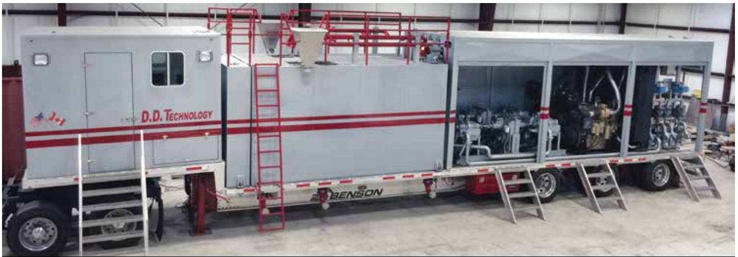
A DDT Quad Pass pumping unit supplies high-pressure water that pushes a patented Pigg through refinery pipelines to remove the buildup of coke.
