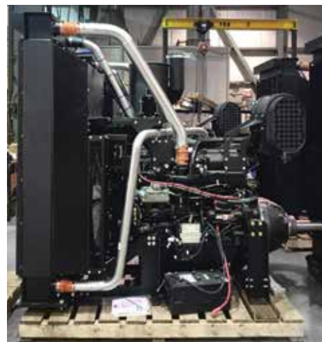
Frontier Power Products supplied DDT with several power units, including this one powered by a John Deere PowerTech Plus 13.5L engine.
